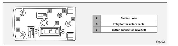
**1** • Prepare the output for the electric and unlock cables, respecting the preset sapaces on the switch box. Use the 3 fixation holes to fix the switch box to the wall.
