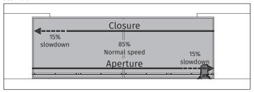
The control board automatically sets a slowdown in opening and closing equal to
